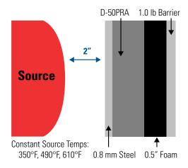
TUFCOTE™ D Series foam is very effective at reducing thermal loads in areas with high heat sources where little space is available.
