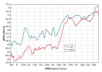
In acoustic system level testing, sound pressure is measured against speed to determine how engine load change impacts the driver. This test can help pinpoint which components are producing sound at which speeds, to better understand the overall acoustic issues of the vehicle.
