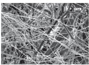
The thicker polyester fibers add loft, strength and stability, while the extremely fine polypropylene fibers allow for high-energy absorption without adding weight.
