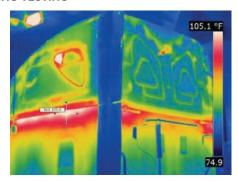
Thermal imaging tests allow our technicians to find the weak points in a cabin when exposed to different conditions. They can then find where heat leaks may occur and construct a plan for insulation.
