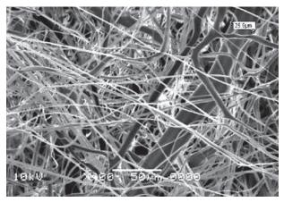
The thicker polyester fibers add loft, strength and stability, while the extremely fine polypropylene fibers allow for high-energy absorption without adding weight.
