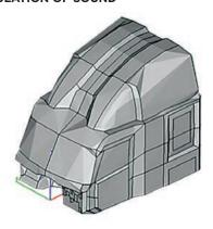
Vibroacoustics Simulation Software (VA One) is used to predict in-cabin sound pressure levels using Statistical Energy Analysis (SEA).
