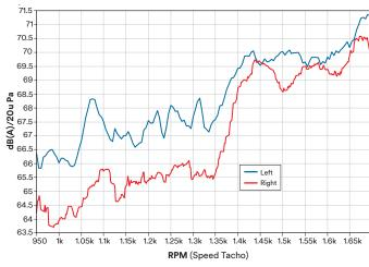
In acoustic system level testing, sound pressure is measured against speed to determine how engine load change impacts the driver. This test can help pinpoint which components are producing sound at which speeds, to better understand the overall acoustic issues of the vehicle.
