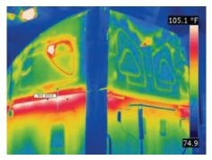
Thermal imaging tests allow our technicians to find the weak points in a cabin when exposed to different conditions. They can then find where heat leaks may occur and construct a plan for insulation.
