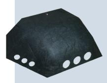
Thin and lightweight 3M™ Thinsulate™ insulation material is made of fine microfibers that trap air and block heat loss. Custom designed parts can be molded in a single piece for faster, easier installation — and to reduce leakage from gaps. The three-dimensional parts are stiff enough to be self-supporting while filling the application cavity.
